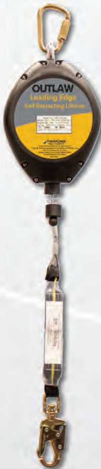
XR-50LEG Leading Edge SRL 50' galvanized cable only #354-4 (1" opening) steel carabiner #49 (3/4" opening) locking snap Class "B" SRL
